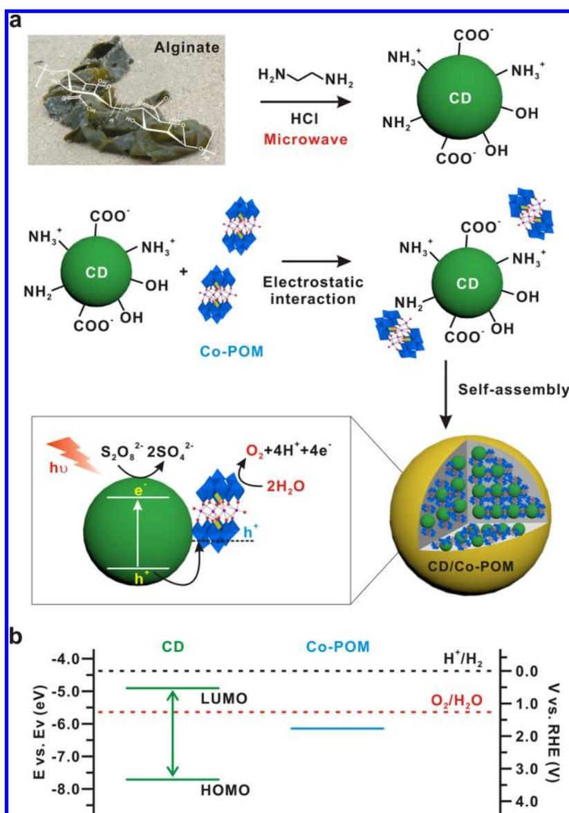
**Figure 1.** (a) Preparation of supramolecular hybrid CD/Co-POM structure for photocatalytic water oxidation. (b) Band diagram of CD and Co-POM.
